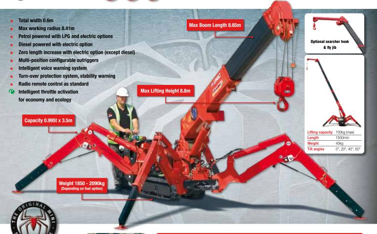
The URW-095 is just 0.6m wide and designed specifically for interior access and benefits from class-leading heavy lifting
