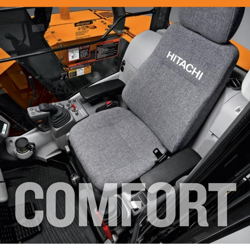
Low-effort joysticks, a highly efficient HVAC system, and plenty of storage space maximize comfort and convenience. A comfortable, mechanical suspension fabric-covered highback seat provides plenty of travel, sliding together or independent of the joystick console. Automatic, high-velocity bi-level climate-control system with automotive-style adjustable louvers help keep the glass clear, the cab comfortable, and the operator productive.
