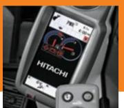
Multi-language LCD monitor and rotary dial provide access to a wealth of info and functions. Just dial and tap to check diagnostic codes, monitor maintenance intervals, set cab temperature and more.
