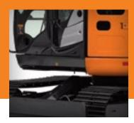
Reinforced D-channel side frames provide maximum cab and component protection.
