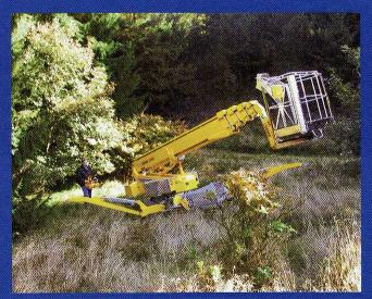
Before reaching the maximum incline limits, a tilt alarm is activated. When there is a doubt about the gradient, place the lift on stabilizers to reach a safe position.
