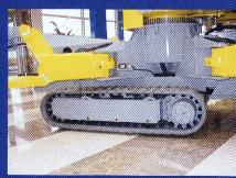
The surface is protected by non-marking tracks and the surface pressure is reduced to only 6 N/cm<sup>2</sup>.
