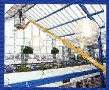
The basket mounting forms a "fly" boom on the top boom section which gives increased outreach over obstacles.
