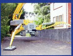
The specially designed stabilizers provide easy lift deployment.
