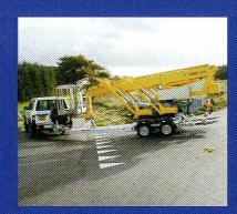
Transport on a purpose designed trailer. Up to type 2200, the total weight is less than 3500 kg.
