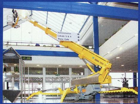
Battery operated lifts are used indoors to avoid noise and emmissions.
