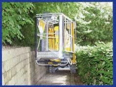
The transport width is reduced to 1.1 m when the basket is rotated.
