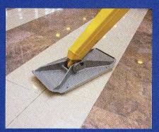
The lifts are equipped with large base plates (1250 cm<sup>2</sup>). This provides a spread of the maximum stabilizer load of 25 kN (maximum 20 N/cm<sup>2</sup>).
