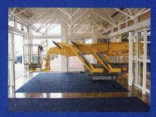
Due to a transport width and -height of only 1.10/1.98 m entry through most doorways and arches is possible.
