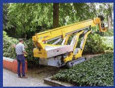
The diesel power pack provides a maximum gradability up to 40 % (21.8°), in an environment where lift deployment is possible.
