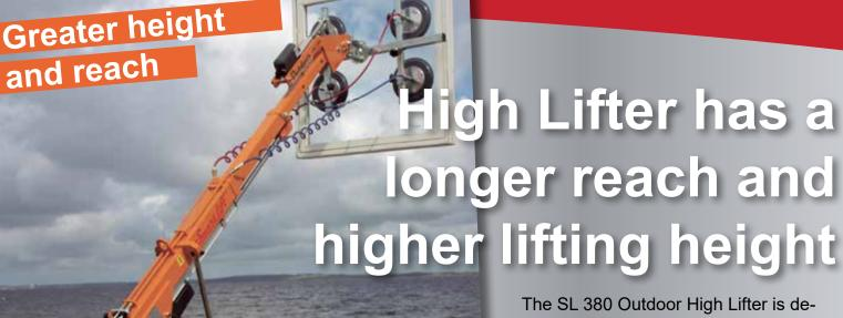
The SL 380 Outdoor High Lifter is designed for jobs that require additional reach and lifting height. The High Lifter easily handles jobs across basement shafts and flower beds and replacement of windows in end walls etc.
